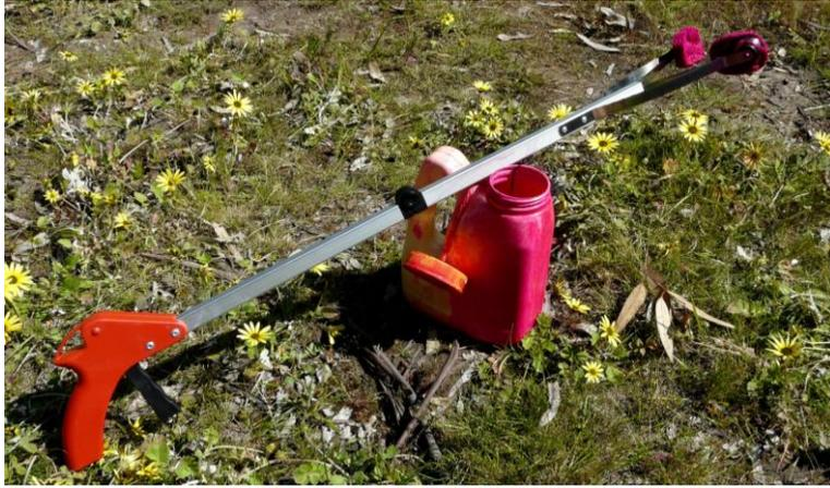
Photo 1. A weed-wiping tool adapted by members of HFNC
